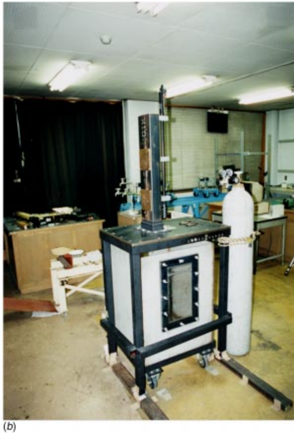
Fig. 1 (a) Experimental setup for optical observation of high-speed water entry. (b) Photograph of the experimental setup for water entry tests
